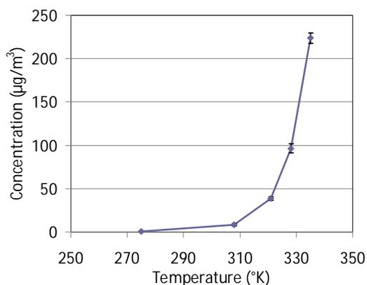
**Figure 2.** Steady state concentrations of DEHP emitted from vinyl flooring in FLEC as a function of temperature. Error bars is 95% confidence intervals.
