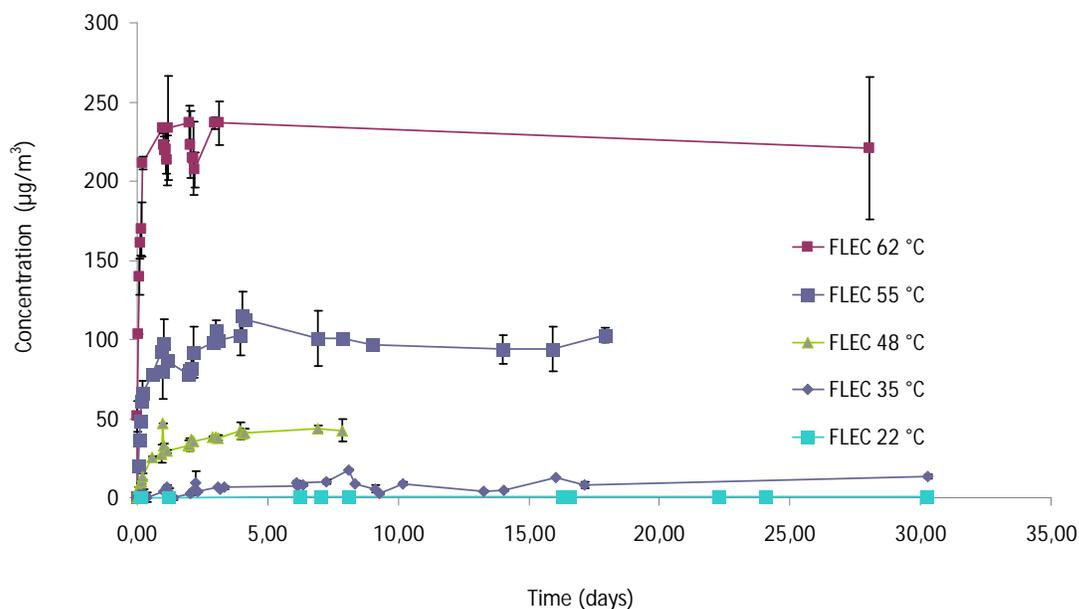
**Figure 1.** Concentration versus time data for emission of DEHP from vinyl flooring in FLECs at five different temperatures. The error bars indicate the standard deviation for duplicate sampling.
